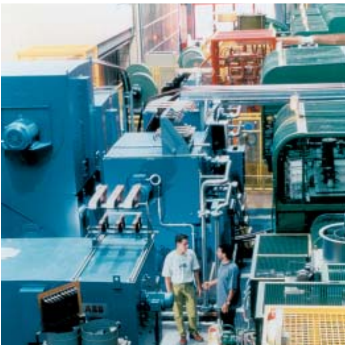
View of ABB's test machines at the drive factory in Switzerland. Every ACS 1000 drive will undergo a load test driving a medium voltage motor with load, in order to subject it to 'real life' operating conditions, before shipping it to customer's site.
